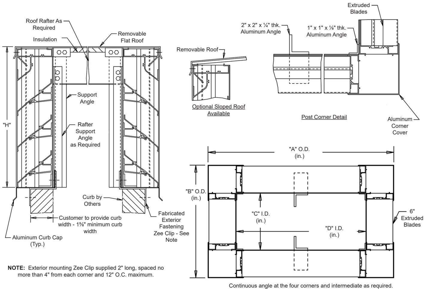
**NOTE:** Exterior mounting Zee Clip supplied 2" long, spaced no more than 4" from each corner and 12" O.C. maximum.
